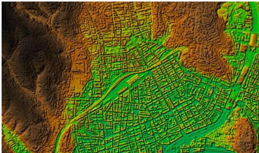
Figure 82: Simulated CO3D DSM over Nice (downtown), France, based on Pleiades-HR data © CNES 2020
