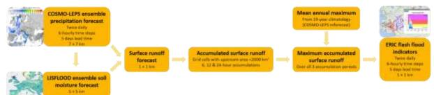
Figure 88: The ERIC flash flood forecasting modelling chain
