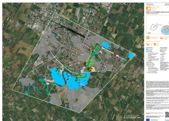
Figure 1: Example of flood product provided by Copernicus EMS (EMSR664, AOI04). Flood delineation is available outside of settlements, but could not be extracted or digitized inside urban areas due to their geometry and other properties.
